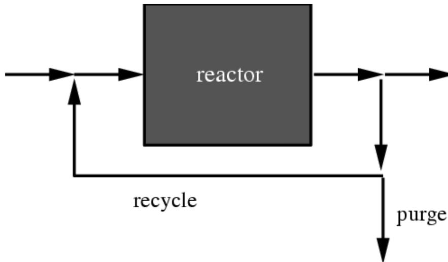
This is common with multi-phase systems where only 1 phase is either removed or recycled (i.e., if one recycles catalyst pellets, but adds "make-up" fresh catalyst a purge will be needed to discard some "spent" catalyst).
