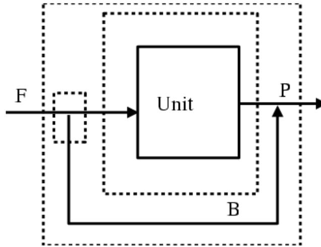
This practice is far less common than recycle, but may be used if your ultimate goal is a material with properties "in-between" the untreated reactant and the process outlet product.
